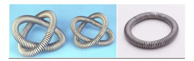
Garter Springs are helical coil springs whose ends are connected together to form a circular shape to provide a strong Radial Force. Compression garter springs exert outward radial forces, while extension garter springs exert inward radial forces.
